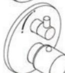
Thermostatic mixer with shut off unit
