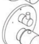
Thermostatic mixer with shut off and
